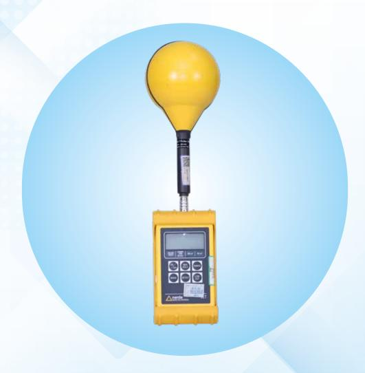
Extremely precise equipment to assess electronic and electrical equipment related to human exposure restrictions for electric, magnetic and electromagnetic fields.
